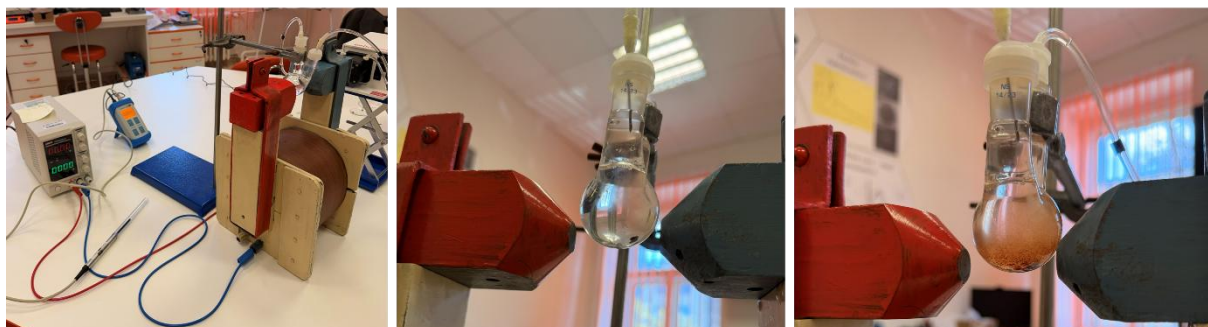
Figure 2 Experimental setup designed to investigate deeper penetration of \text{Fe}_3\text{O}_4@\text{SiO}_2 nanoparticles into a blood clot under the influence of an alternating magnetic field. The setup included a coil system for modulation of the magnetic field strength. A model blood clot was placed in physiological medium inside the experimental vessel, in the presence of a magnet. Magnetic nanoparticles accumulated in the clot region, while the alternating magnetic field was intended to promote oscillation of the magnetic cores and facilitate deeper nanoparticle penetration into the clot structure.
