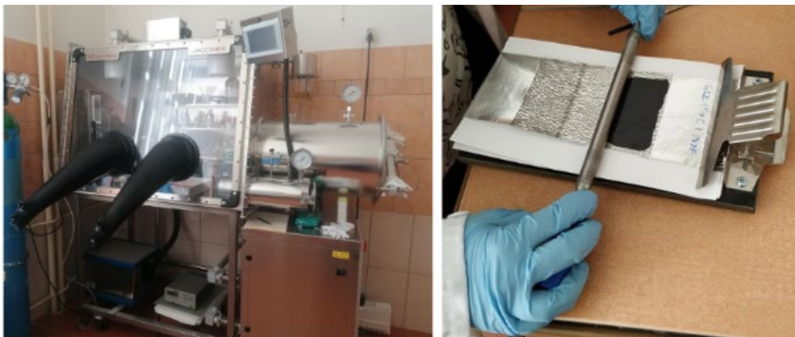
Figure 1(Left) Argon-filled GloveBox used for assembly and handling of oxygen-sensitive battery components. (Right) Photo of sulfur-carbon composite slurries and their coating onto aluminium foil current collectors.
