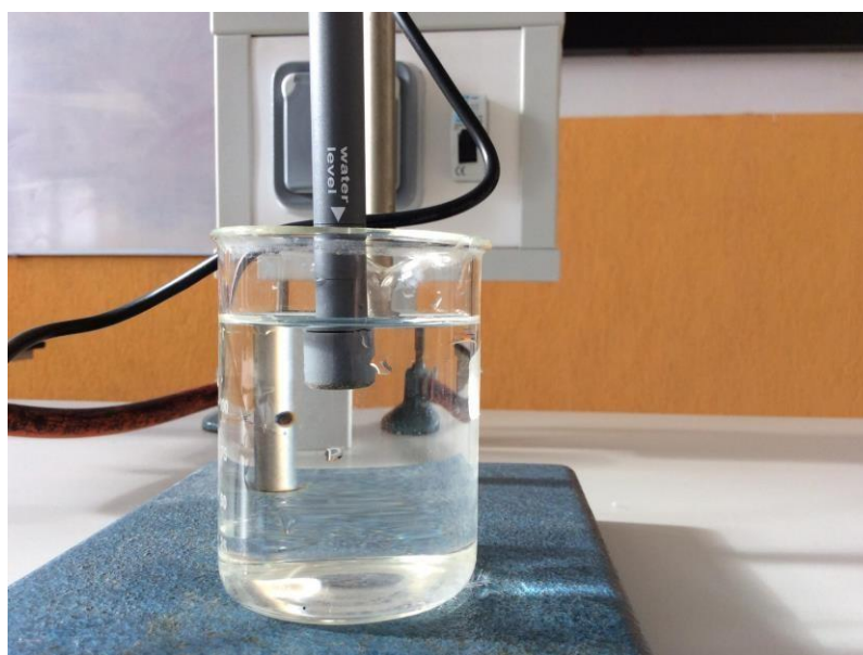
Fig. 16. Incorrect immersion of NO 3 - sensor into the sample (white reference points are not submerged in the solution)
