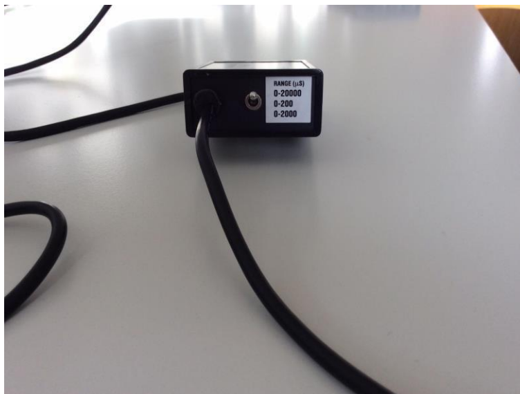
Fig. 6. Measurement Range Switch - Use it only during calibration
