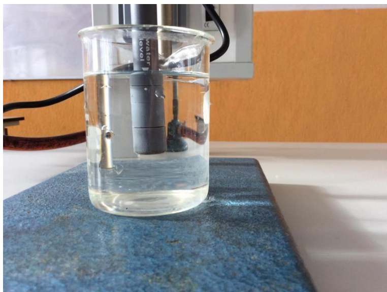
Fig. 15. Correct submersion of the sensor into the sample
