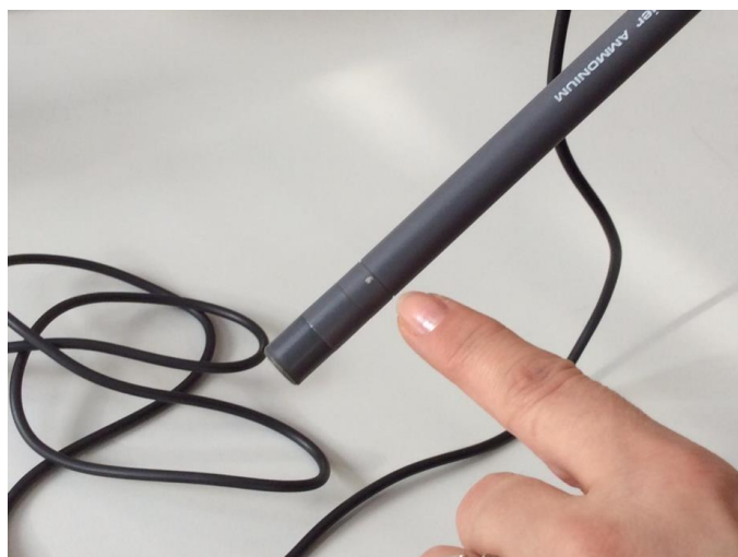
Fig. 18. The white reference dot near the electrode tip. When measuring a sample, it is sufficient to submerge the sensor just slightly above this point.
