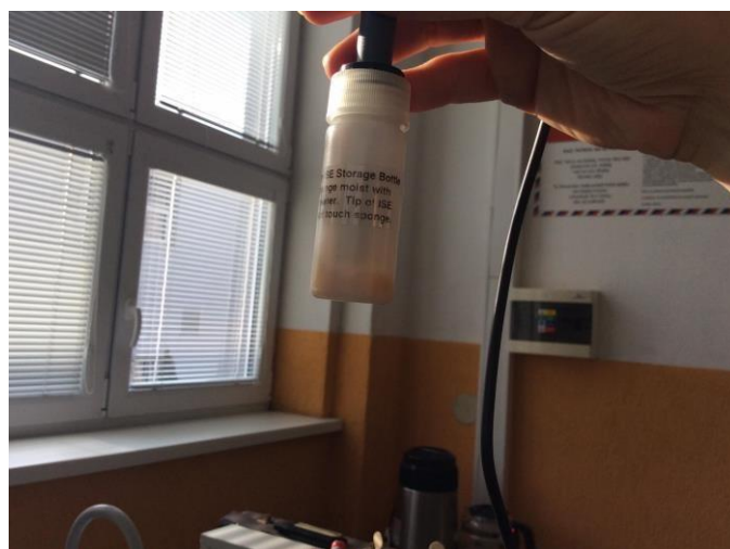
Fig. 20. Properly stored electrode in the storage bottle (the lower edge of the sensor does not touch the sponge, which is moistened with distilled water).
