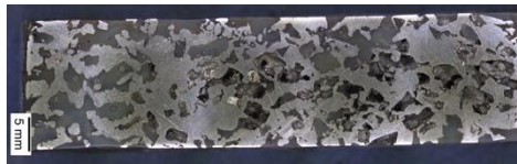
Fig. 1 PA6 – AlSi12 foam hybrid structure under 0.7x magnification
