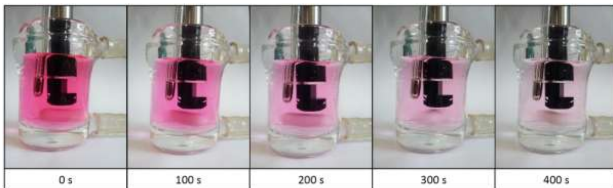
Figure 1. Pictures of the reaction mixture at different times under the following conditions: c(\text{AP}) = 10 \mu\text{mol/L} ; c(\text{H}_2\text{SO}_4) = 0.9 \text{ mol/L} ; c_m(\text{Cr}^{6+}) = 0.5 \text{ mg/L} ; t = 60 \text{ }^\circ\text{C} .
